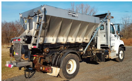
One of DPW's Salt Trucks with a capacity of 10 tons of rock salt.
